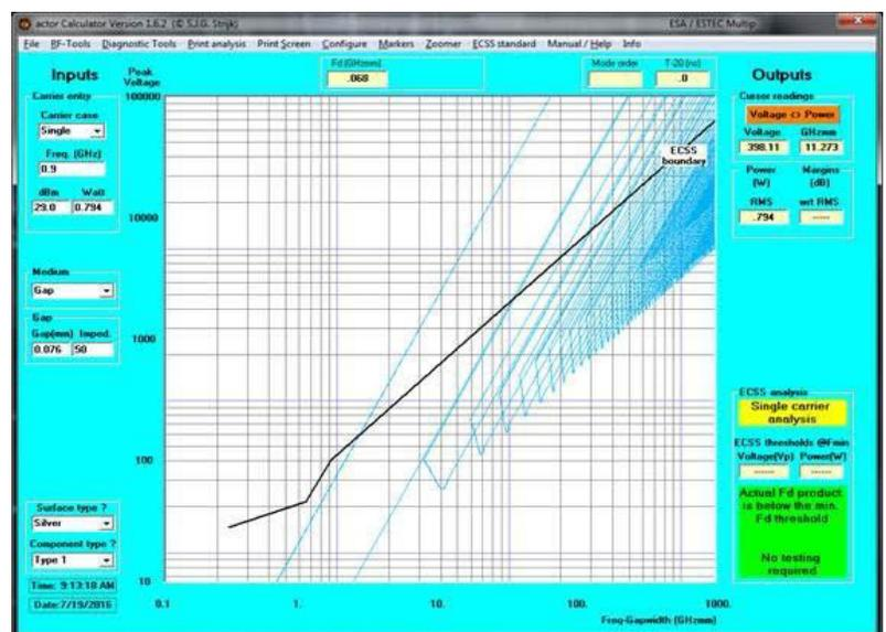
*Highly specialized multipactor predictive tools enable filter and other RF passive component designs that ensure a long life of operation without concern of this breakdown threat.*
